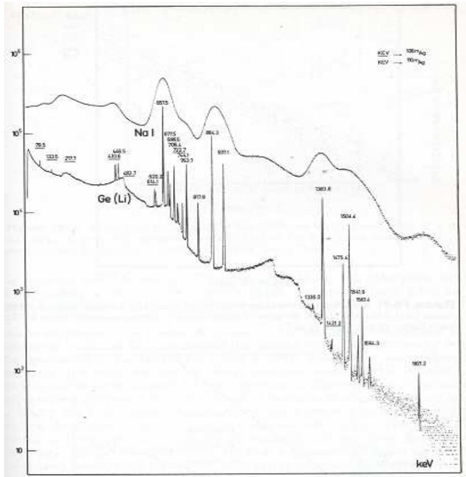
Figure 1.1 Comparative pulse height spectra recorded using NaI and Ge(Li) [1]
