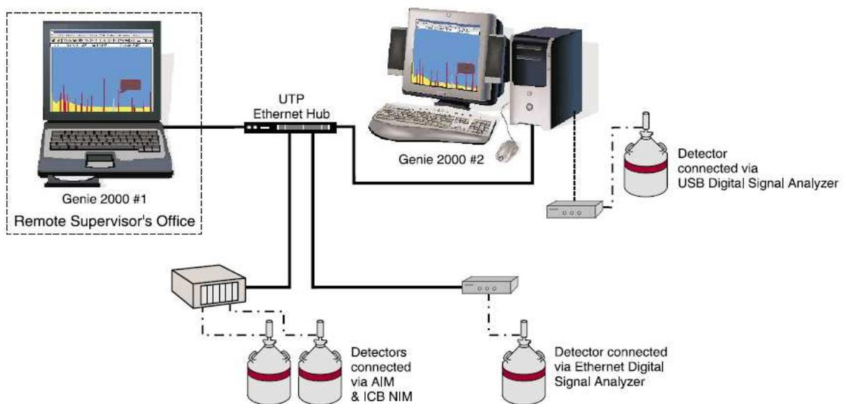
Figure 3.2 Diagram of Multiple Genie 2000 Network.[14]
