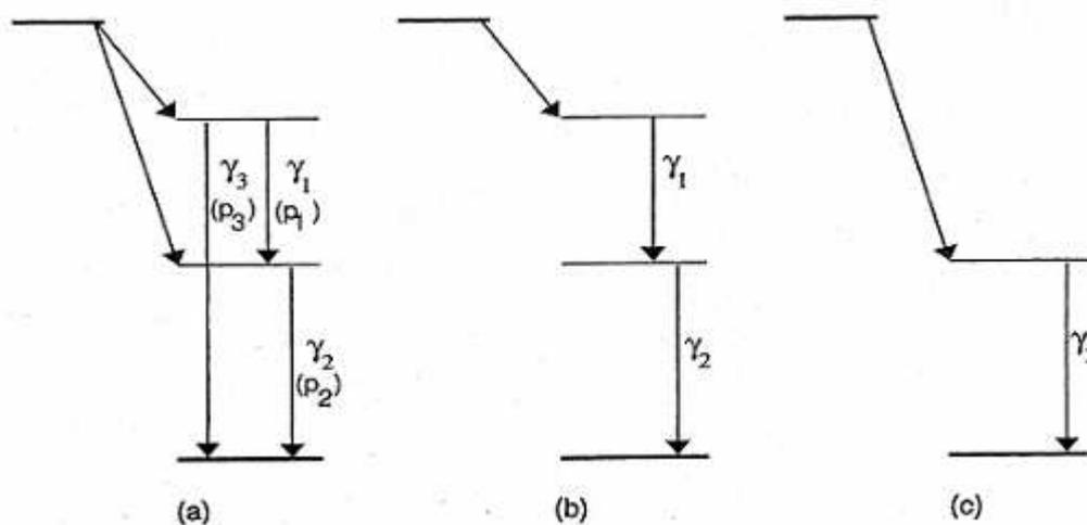
Figure 2.10 Simple illustrative decay scheme liable to true coincidence summing [2]
