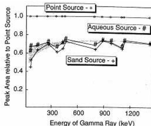
Figure 2.9 Relative peak areas for sources of different geometry and density [10]
