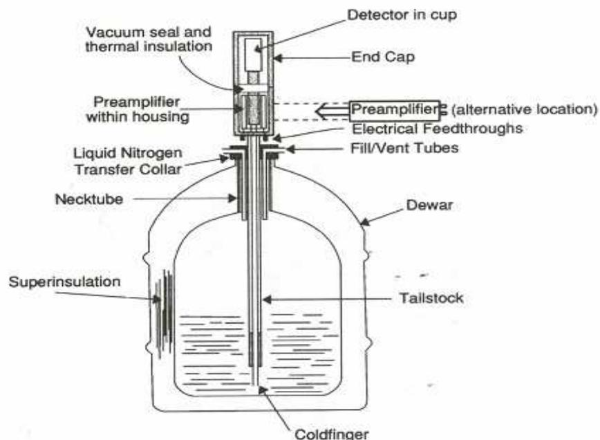
Figure 1.4 A typical germanium detector, cryostat and liquid nitrogen reservoir [3]
