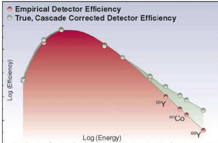
**Figure 3.5** Comparison of Cascade Corrected to Empirical Efficiency. [15]
