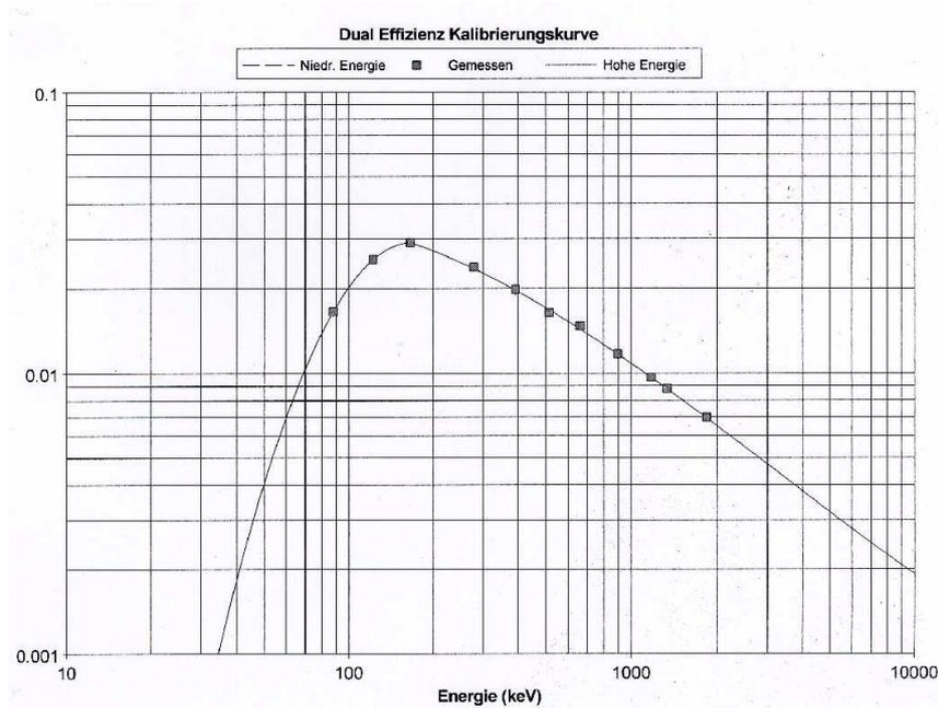
Figure-1.9 Full peak energy calibration curve for a Marinelli Beaker
