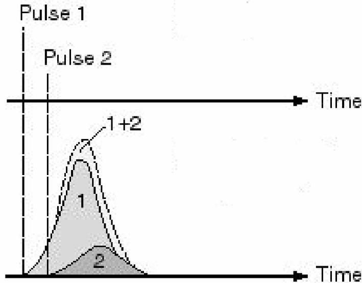
Figure 2.1 Registered pulse shapes resulting in coincidence summing [6]
