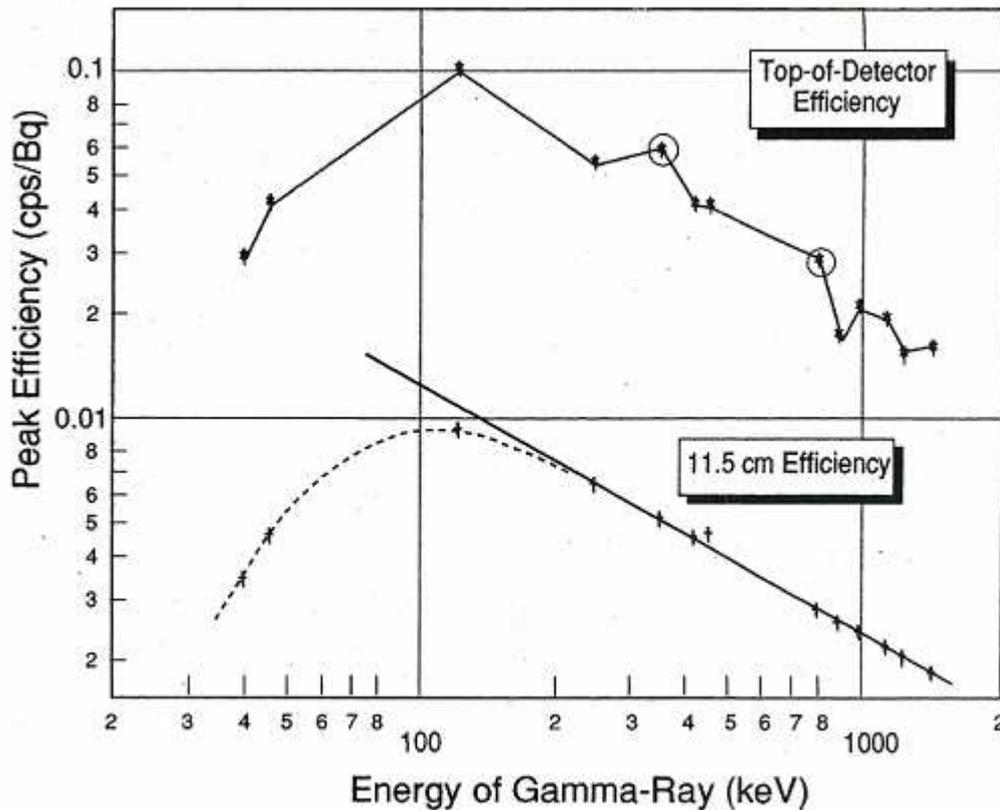
Figure 2.2 Efficiency curves on top of and at 115 mm from the detector end cap using Eu-152 [7]
