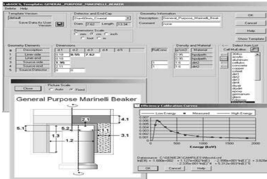
**Figure 3.6** LabSOCS Calibration Software is launched, used for data entry, and then generates the Efficiency Calibration Curve[16].
