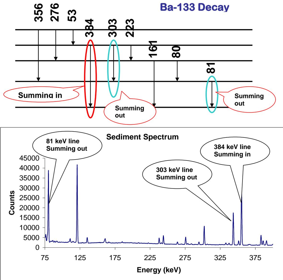
Figure-3.1 The decay scheme and a spectrum of Ba-133 showing the summing-in summing out peaks
