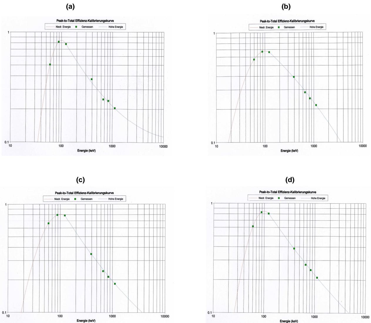
**Figure 4.2** The P/T calibration curves for the four detectors in log-log scale
