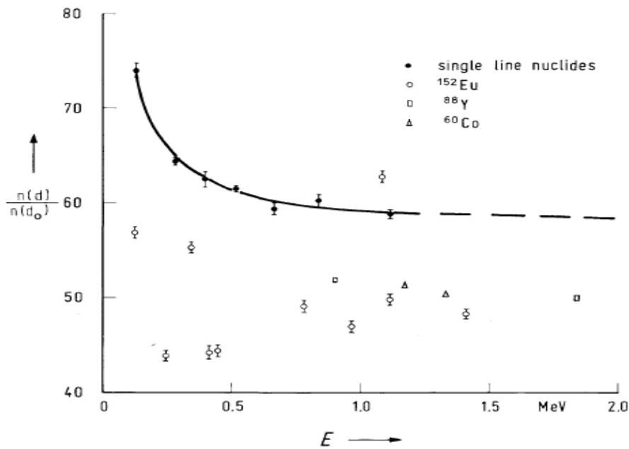
**Figure 2.6** Ratio of count rates in the full-energy peaks for a point source positioned at a short distance  $d$  and a large distance  $d_0$ . The solid line has been drawn by hand.[1]
