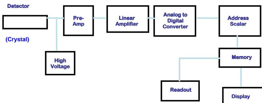
Figure 1.6 A simple schematic electronic system for gamma spectroscopy
