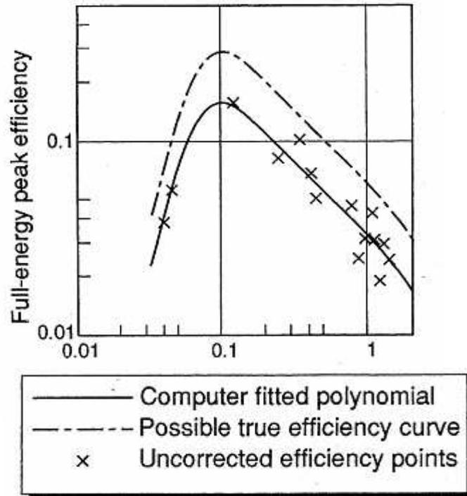
**Figure 2.8** The efficiency curve constructed using a 'best fit' computer program [10]
