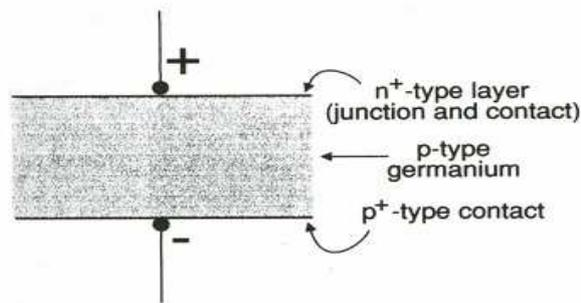
Figure 1.2 The basic construction of germanium detector. [1]
