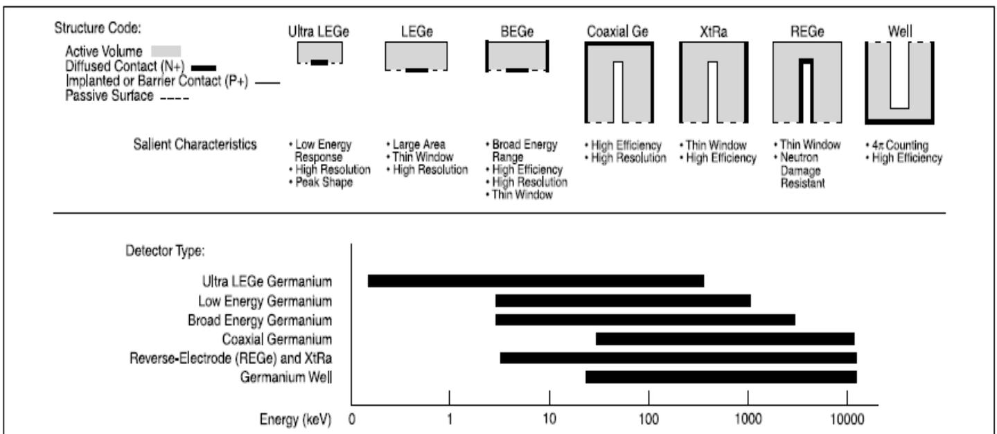
Figure 1.3 Configuration of detector generally available together with the used energy range [3]
