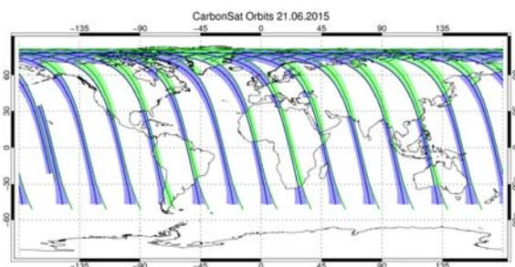
**Figure 5:** CarbonSat orbital coverage (swath width 500 km). Green indicates the coverage obtained in nadir mode over land. Blue indicates the coverage in sun-glint mode over water. The orbits are for daylight for midsummer in the northern hemisphere.
