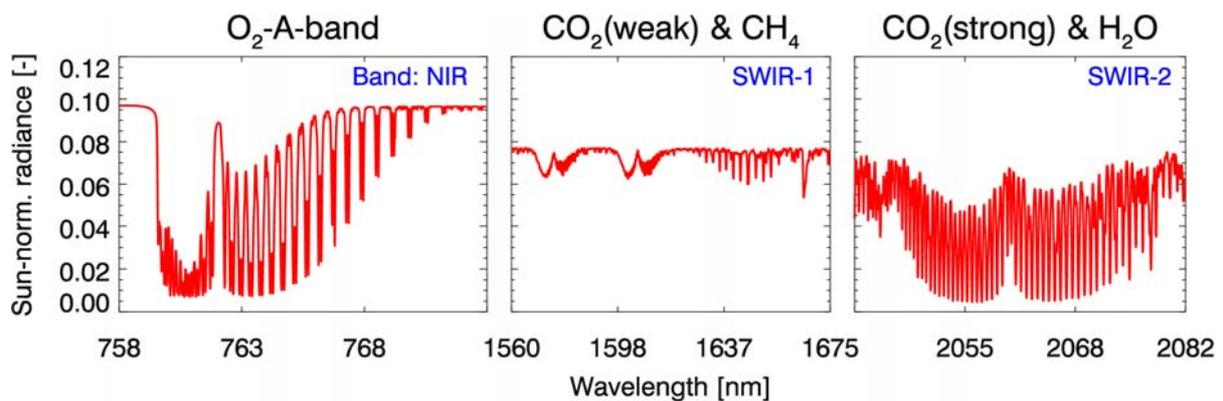
**Figure 8:** CarbonSat's spectral bands covered by the Imaging Spectrometer.
