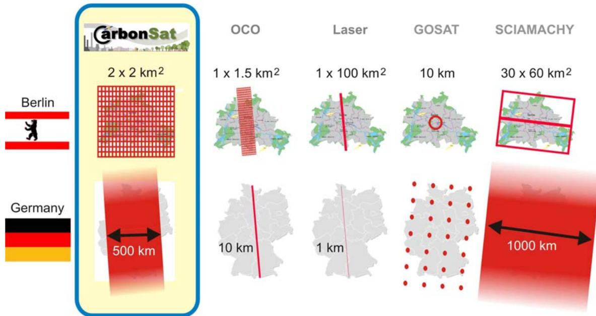
**Figure 4:** Examples of the spatial resolution of CarbonSat (top row; as illustrated the city of Berlin) and orbital coverage (bottom row; as illustrated for Germany) compared to a potential LIDAR instrument, the existing GOSAT and SCIAMACHY missions as well as to the planned OCO-2 mission.
