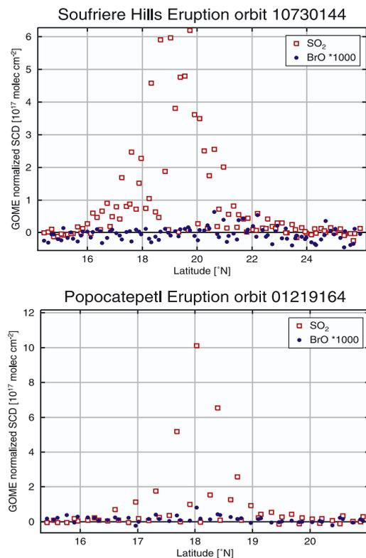
**Figure 2.** Comparison of the GOME  $\text{SO}_2$  and corresponding BrO normalized slant column densities for the Soufrière Hills volcano on 30th July 2001 (top) and the Popocatepetl volcano (bottom) on 19th December 2000.
