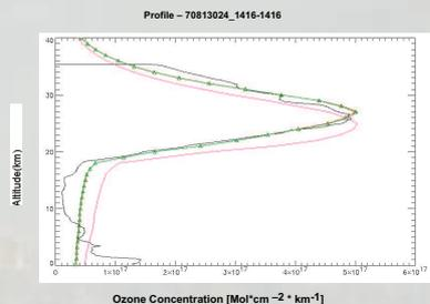
Figure 2: Ozone vertical profiles for a GOME ground pixel extracted for the 13<sup>th</sup> of August 1997. The black, green and pink curves indicate the sonde, FURM and a priori profiles respectively.
