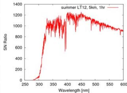
Figure 3: Example of Signal-to-Noise ratio calculated by using the CCD sensor specification with a spatial resolution of 5km and a time resolution of 1hr, which is currently discussed for a Japanese geostationary instrument. Shot noise is assumed to be the main component of noise.
