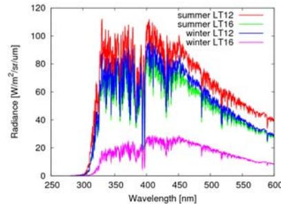
Figure 2: Earth's atmospheric radiance at satellite calculated by SCIATRAN for summer and winter at LT12 and 16
