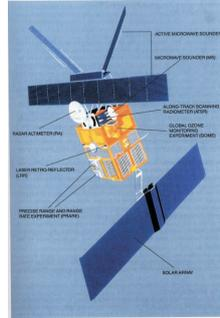
The *Global Ozone Monitoring Experiment* (GOME) is a grating spectrometer observing light scattered back by the atmosphere and reflected from the ground in a near nadir viewing geometry. GOME covers the spectral range of 240 to 790 nm with 0.2 - 0.4 nm resolution. The spatial resolution is 320 x 40 km<sup>2</sup>, resulting in a global coverage every three days. The instrument has been launched on ERS-2 in a polar sun-synchronous orbit in April 1995, and is operational since fall of that year.
