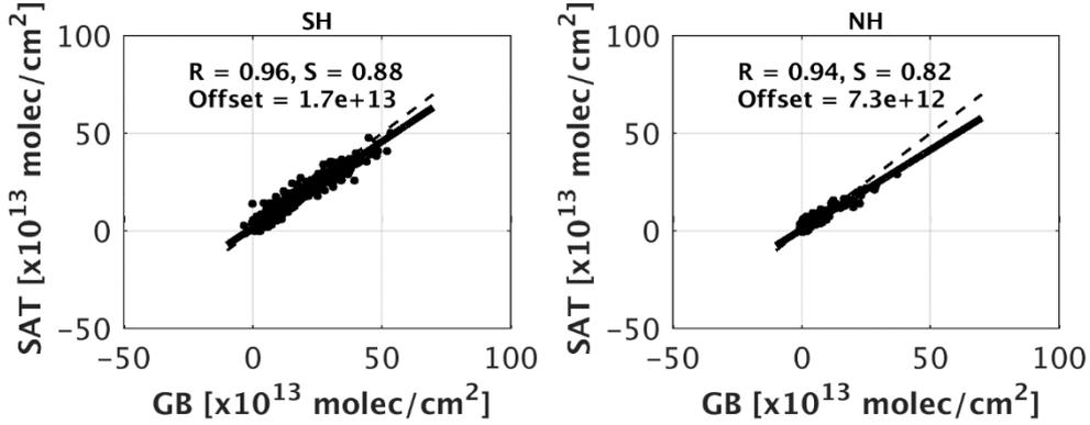
Figure 8.7: Scatter plot of TROPOMI and ground-based data over all stations, during activated months, separated per Hemisphere. Southern Hemisphere on the left panel, Northern Hemisphere on the right panel.
