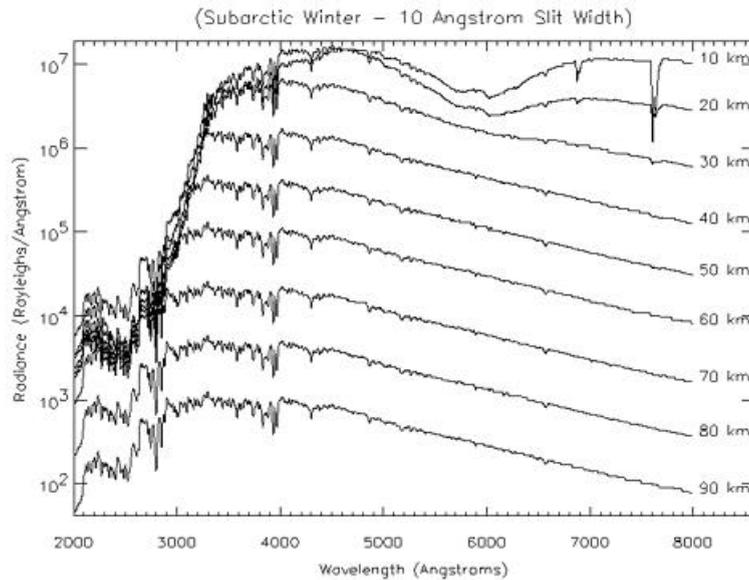
Fig. 2: Typical on-orbit limb spectra that will be measured with OSIRIS. These spectra were calculated using the MODTRAN code for high latitude winter conditions and convolved with a 10 Angstrom slit function (Picture by Univ. Saskatchewan).
