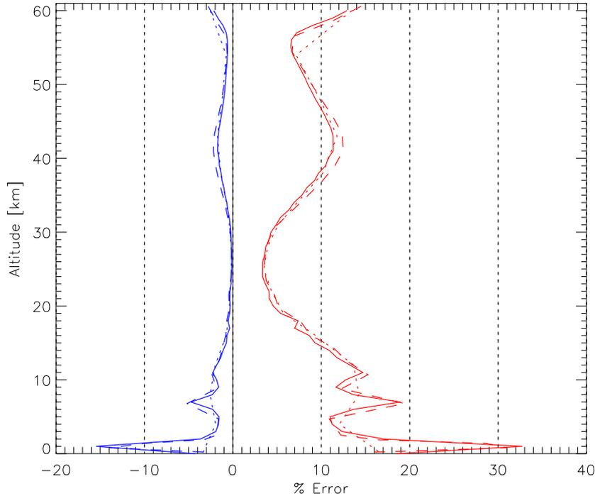
Figure 2: Comparison of Bias (blue) and standard deviation (red) for 61 (solid), 34 (dashed) and 16 (dotted) output neurons corresponding to the heights given in Table 2.
