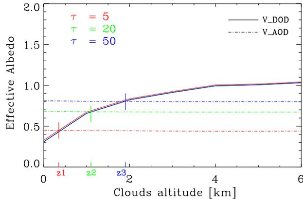
Fig. 2: Determination of the effective albedo and cloud-top-height for different optical cloud depths
