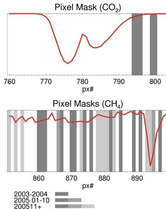
Figure 1. Detector pixel masks used in WFMDOAS2.0. Due to proceeding detector degradation in channel 6+ three different static pixel masks dependent on the analysed time period are used for the  $CH_4$  retrieval.
