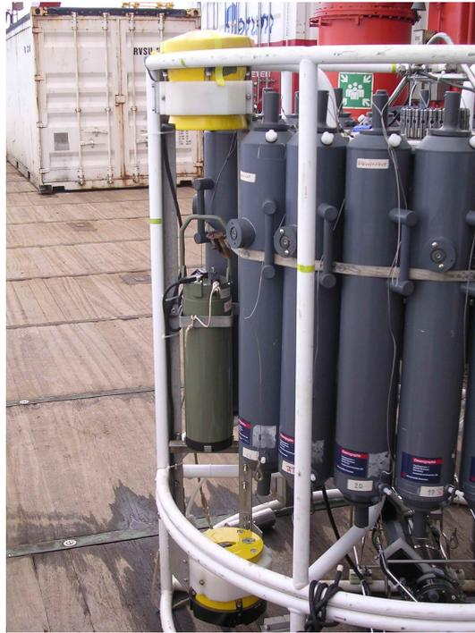
Figure 3.2: A photo of CTD-ADCP instrument package. The two yellow ADCPs are attached to rosette frames in opposite direction (one upward and the other downward). Photo is given by O. Bislich.
