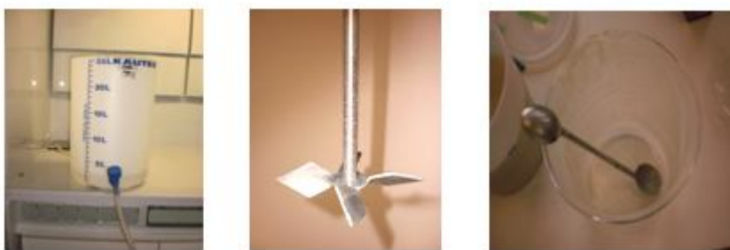
Figure 23: Left picture: 25 Liter container, Center picture: Material attached on the stirrer, Right picture: Material attached in beaker walls after the addition of glue and the transfer into a Marinelli beaker.
