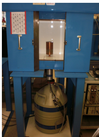
Figure 13: Typical germanium detector with lead shielding attached to liquid nitrogen reservoir (bottom).
