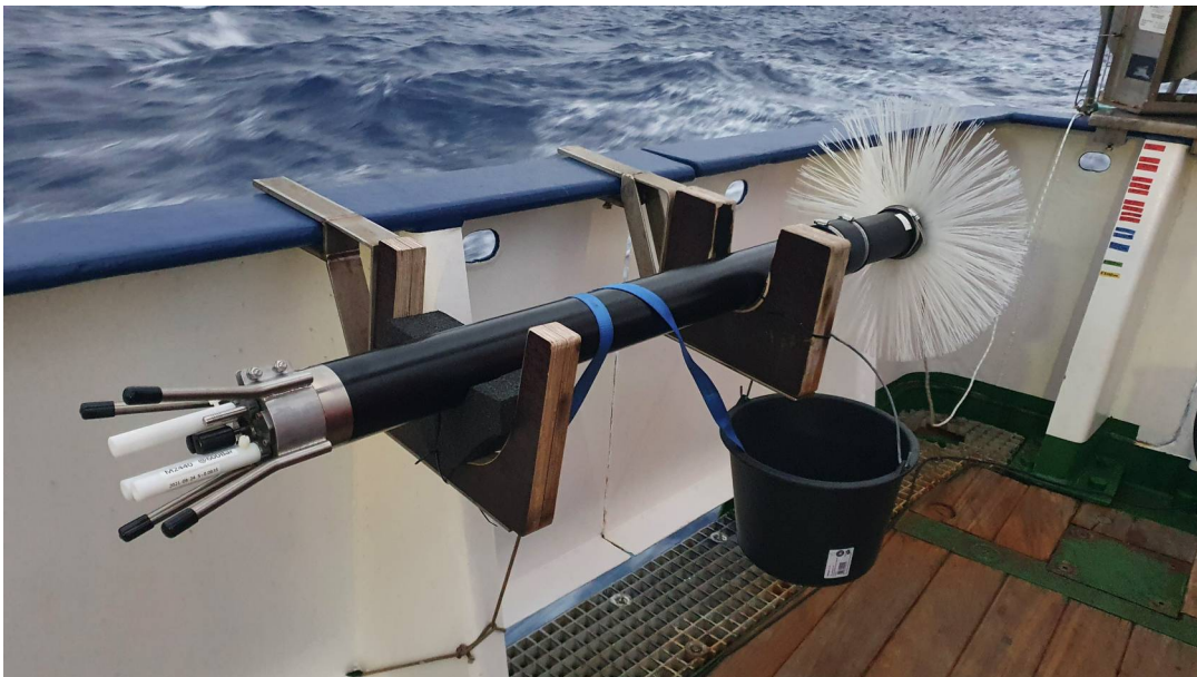
Figure 6: The Vertical Microstructure Profiler (VMP) secured on a deck of the Meteor Research Vessel. The temperature and shear probes are protected with white protection cases.
