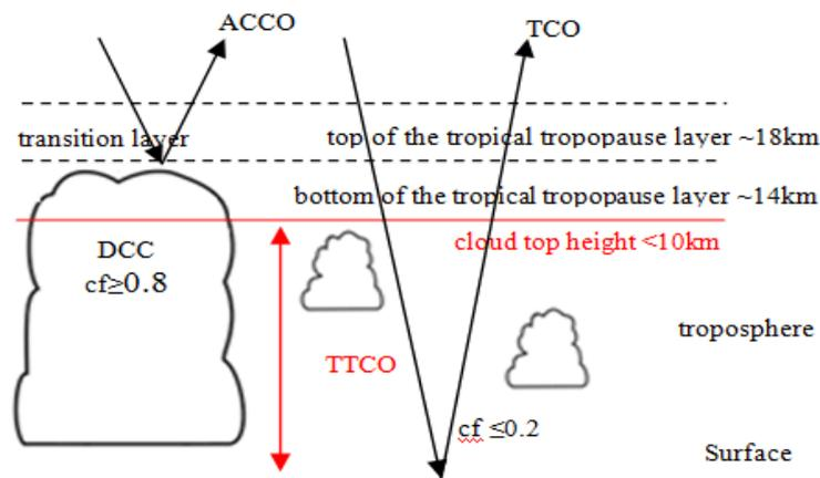
**Fig. 1** Illustration of the Convective Clouds Differential (CCD) technique. DCC are the deep convective clouds, cf is the cloud fraction, ACCO is the above cloud column of ozone, TCO is the total column of ozone and TTCO is the tropical tropospheric column of ozone.
