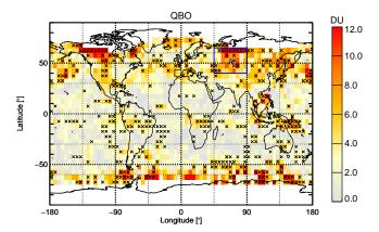
**Figure 8.** Same as Fig. 7 but for QBO. Here the maximum response is derived from the sum of the two QBO terms in the regression. The regions with crosses indicate grid boxes where at least one of the QBO regression coefficients is statistically significant to  $2\sigma$ .
