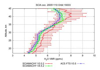
**Figure 3.** Example of  $H_2O$  VMR profiles. Red: previous product (V2.0.2) from Noël et al. (2010). Green: current product (V4.5.2). Blue: collocated profile from ACE-FTS V3.5.
