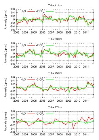
Figure 8. Time series of SCIAMACHY water vapour and methane anomalies at different altitudes. Methane data have been scaled by a factor of -2.
