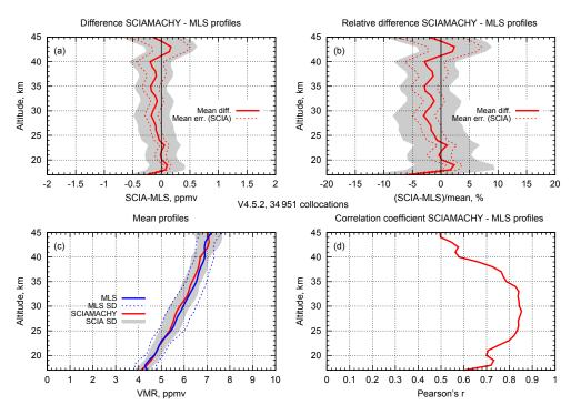
Figure 5. Same as Fig. 4, but for comparison of retrieved SCIAMACHY H<sub>2</sub>O profiles with MLS V4.2 data 2004–2012.
