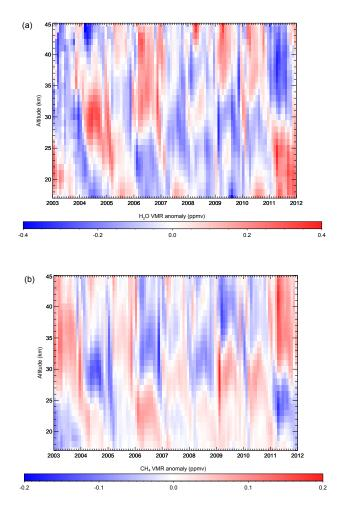
**Figure 7.** Time series of SCIAMACHY  $H_2O$  (**a**) and  $CH_4$  (**b**) monthly VMR anomaly profiles from January 2003 to December 2011. The  $CH_4$  plot is taken from Noël et al. (2016). Note that for these data the same latitudinal dependence as shown in Fig. 6 still applies.
