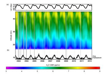
Figure 6. Time series of daily averaged SCIAMACHY  $H_2O$  VMR profiles from August 2002 to April 2012. In the top graph the latitudes of observations as a function of time are shown. Grey vertical bars mask out times of reduced SCIAMACHY performance or missing data. The black curve at lower altitudes shows the average tropopause height.
