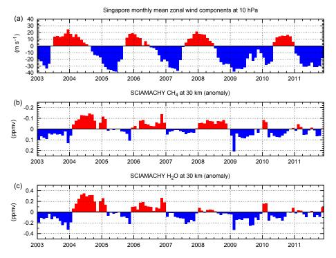
**Figure 9.** Time series of methane and water vapour anomalies at 30 km (**b**, **c**) and Singapore zonal wind at 10 hPa, corresponding to about 30 km (**a**). Note that the vertical axis of the methane data is inverted and scaled differently than for water vapour.
