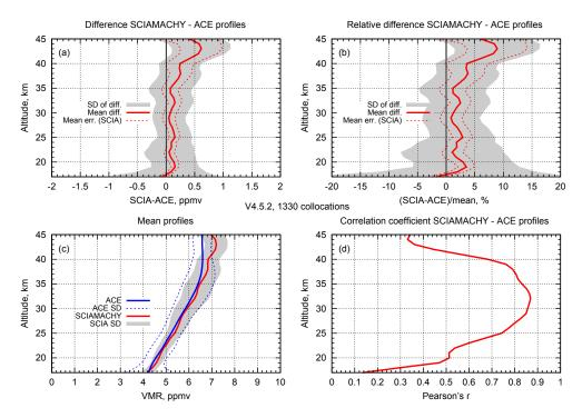
**Figure 4.** Comparison of retrieved SCIAMACHY  $H_2O$  profiles with ACE-FTS data 2004–2012. (a) Mean difference plus/minus one standard deviation (SD) (shaded area) and mean error of SCIAMACHY data (dotted line). (b) Mean relative difference plus/minus one standard deviation (shaded area) and mean relative error of SCIAMACHY data (dotted line). (c) Mean profiles and standard deviations (red: SCIAMACHY, blue: ACE-FTS). (d) Correlation between SCIAMACHY and ACE-FTS data.
