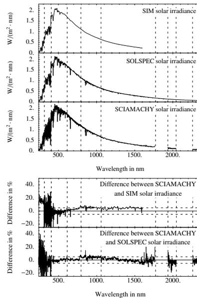
**Fig. 2.** Comparison of solar irradiance measured by SCIAMACHY (2004-03-05) with SIM (2004-05-03) and SOLSPEC spectra. Upper: solar irradiances, lower: difference between SCIAMACHY and other data, SCIAMACHY channel boundaries are marked by vertical dashed lines.
