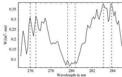
**Fig. 4.** Mg II Fraunhofer line at 280 nm. Wing values are derived from four maxima (outer vertical dashed lines), core values from the h and k doublet emission lines (two center vertical dashed lines).
