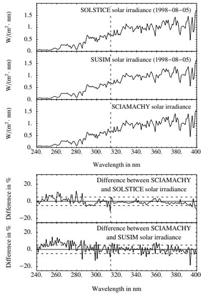
**Fig. 3.** Comparison of solar irradiance measured by SCIAMACHY with data of the UARS instruments SOLSTICE and SUSIM. Upper: solar irradiances, lower: difference between SCIAMACHY and UARS, SCIAMACHY channel boundaries are marked by vertical dashed lines.
