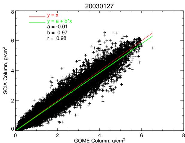
Figure 3. Example for a correlation between GOME and SCIAMACHY water vapour columns.
