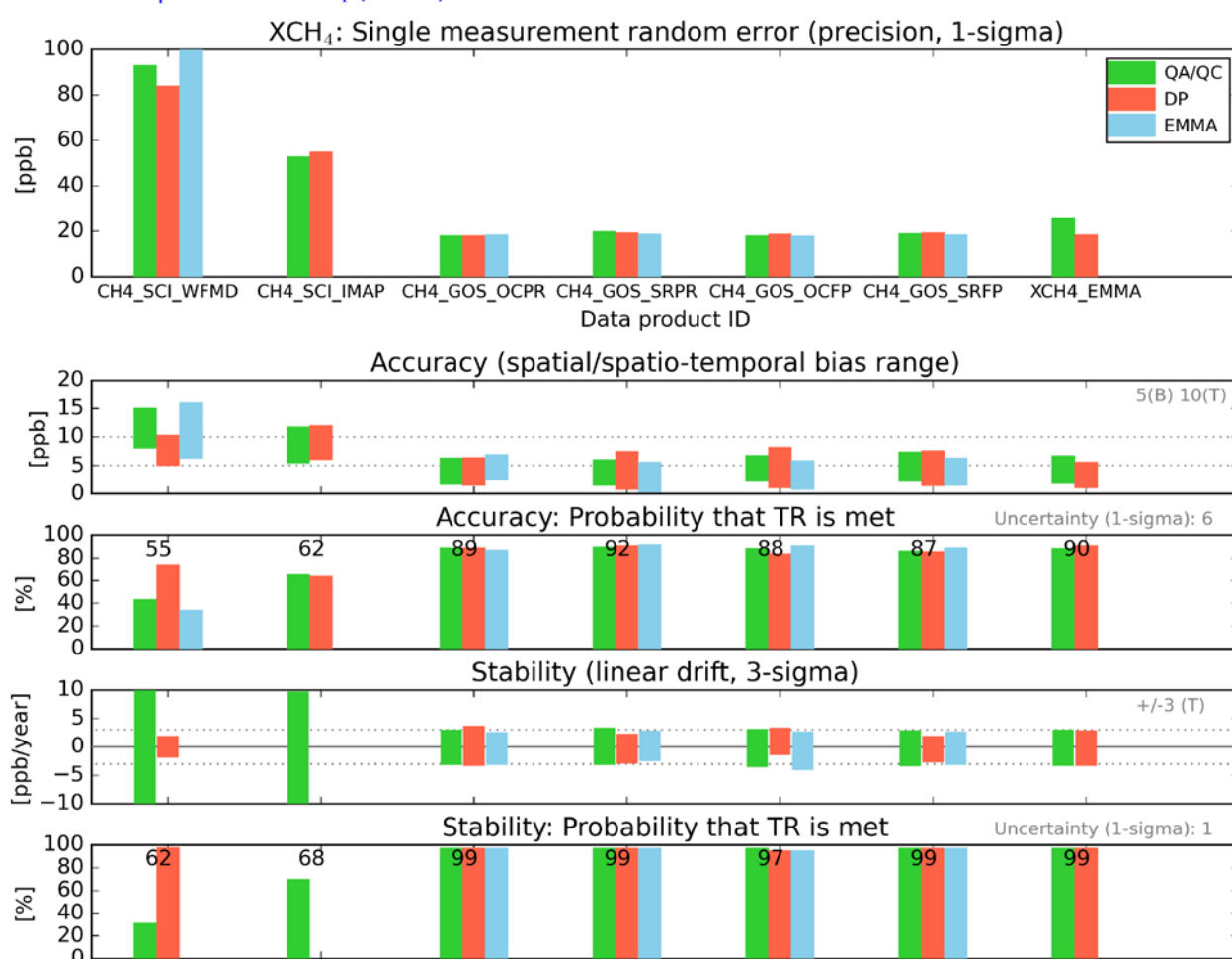
Figure 2 - Overview data quality assessment results for Level 2 XCH 4 data products. The green bars refer to the “Quality Assessment / Quality control” (QA/QC) results as described in this document. The red bars refer to results obtained by the data providers (DPs), as described in separate Annexes (see Sect. 7). The blue bars result from an assessment using the EMMA method (see Sect. 3.2.7). For “Accuracy” and “Stability” also the numerical values for the “Probability that TR is met” are given (computed as mean value if more than one value (bar) exists). Also listed (in grey on the right hand side) is the uncertainty of the reference data as used for the Target Requirements (TR) assessments. The DP values for the “GHG-CCI brokered products” CH 4 _SCI_WFMD and CH 4 _SCI_IMAP are from Buchwitz et al., 2017 .
