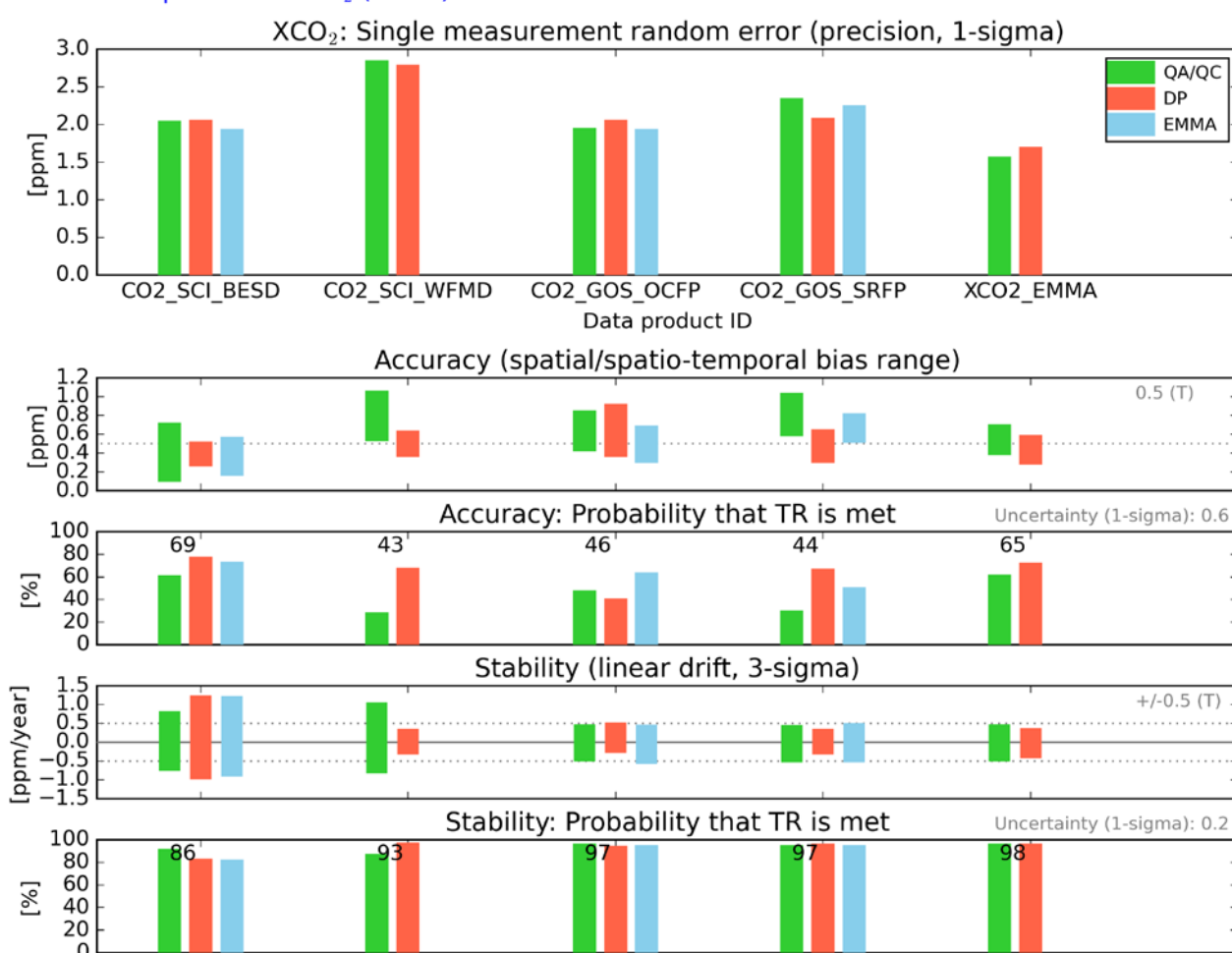
Figure 1 - Overview data quality assessment results for Level 2 XCO 2 data products. The green bars refer to the “Quality Assessment / Quality control” (QA/QC) results as described in this document. The red bars refer to results obtained by the data providers (DPs), as described in separate Annexes (see Sect. 7). The blue bars result from an assessment using the EMMA method (see Sect. 3.1.5). For “Accuracy” and “Stability” also the numerical values for the “Probability that TR is met” are given (computed as mean value if more than one value (bar) exists). Also listed (in grey on the right hand side) is the uncertainty of the reference data as used for the Target Requirements (TR) assessments. The DP values for the “GHG-CCI brokered products” CO 2 _SCI_BESD and CO 2 _SCI_WFM are from Buchwitz et al., 2017 .
