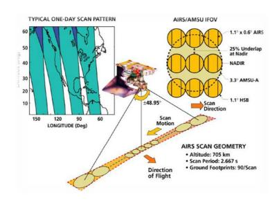
Figure 2: AIRS and AMSU scan geometrics (Jason, 2008).
