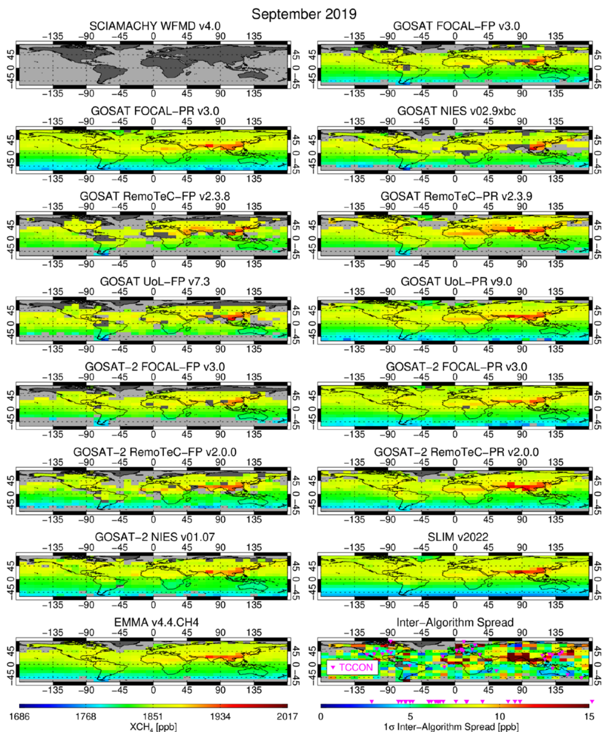
Figure 6: Monthly gridded XCH 4 averages and inter-algorithm spread for the example of September 2019 for EMMA CH 4 .
