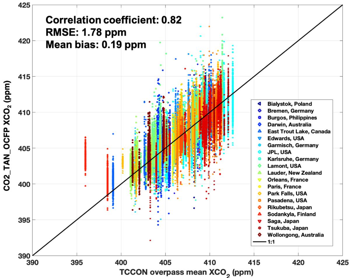
**Figure 2-2.** Comparison of individual retrieved XCO<sub>2</sub> from TanSat with the overpass mean of TCCON XCO<sub>2</sub> for the time period of March 2017 to May 2018 across all 20 TCCON sites. Each TCCON site is given by different colour and symbol. Statistics for mean bias and RMSE (calculated by averaging the bias and RMSE of each site) are given along with the correlation coefficient.
