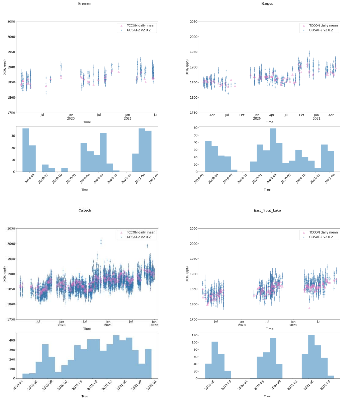
Figure 4.3 Comparison of land single soundings of XCH 4 from the proxy retrieval (blue circles) with co-located TCCON (pink triangles) measurements at all TCCON sites for the period Feb 2019 to Dec 2021. Histograms are also given for each station indicating the number of GOSAT-2 retrievals present throughout the time series.
