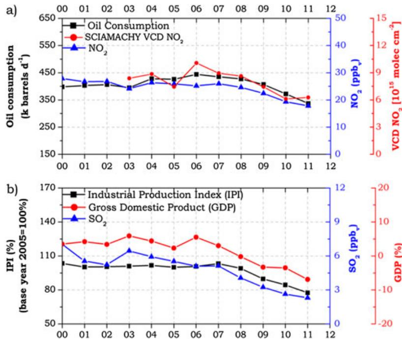
**Figure 3.** The top row (a) presents the annual means of nitrogen dioxide levels (NO<sub>2</sub>) over Athens (blue) compared to the tropospheric SCIAMACHY VCD<sub>NO<sub>2</sub></sub> (red) and the oil consumption per day (black). The bottom row (b) depicts the annual means of sulfur dioxide (SO<sub>2</sub>) levels in Athens (blue), the Gross Domestic Product of Greece (red) and the Industrial Production Index, IPI (black).
