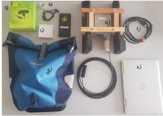
**Figure 3.1:** The components of the setup. a) shows a GPS receiver, b) charging cable for the computer, c) USB lamp, d) power bank, e) Avantes, f) USB data connection between Avantes and computer, h) laptop, and g) bicycle bag or pannier.
