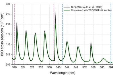
Figure 1. BrO absorption cross-section at 228 K (Wilmouth et al., 1999) used in the DOAS BrO retrieval study. The green line is the BrO cross-section convoluted by the TROPOMI slit function. Pink vertical dashed lines indicate start wavelength ranges and blue lines end wavelength ranges of fitting windows
