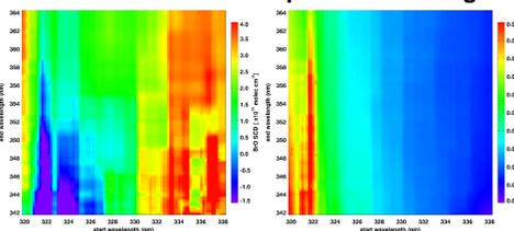
Figure 2. Colour coded means of BrO SCDs (left) and fitting RMS values (right) retrieved over the selected Arctic sea ice region for a BrO explosion event using TROPOMI measurements at different wavelength intervals
