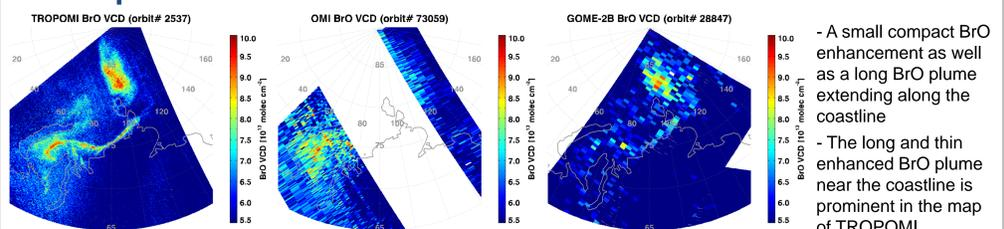
Figure 8. BrO geometric vertical columns observed over the Arctic sea ice region on 10 April 2018 by TROPOMI (left), OMI (middle) and GOME-2B (right)
