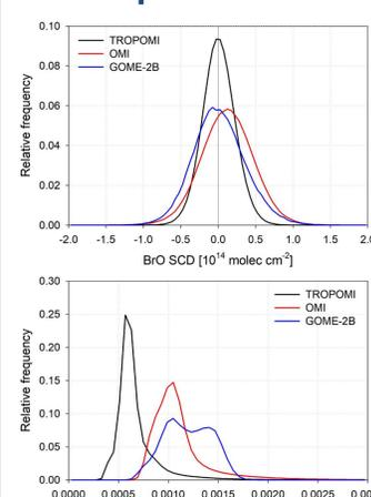
Figure 6. Distribution of BrO SCDs and fitting RMS values over a clean equatorial Pacific region (10°S-10°N, 150-260°E) for April 2018
