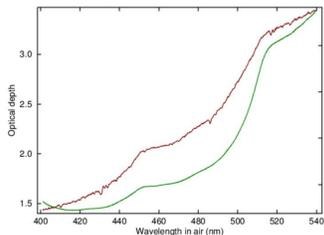
Fig. 4: Blue: Differential VRS cross-section simulated using SCIATRAN [3]. Red: Diff. VRS cross-section retrieved from MAX-DOAS measurements.
