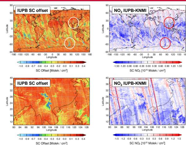
Fig. 4: Left: Fit factor of intensity offset correction in IUPB retrieval (circles indicate enhanced intensity offset not caused by VRS). Right: NO<sub>2</sub> slant column difference between IUPB and KNMI. Global maps (top) and zoom-in over China (bottom). Data from 02 Feb 2005.
