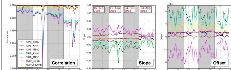
Fig. 2: Correlation coefficients, slope and offset from a linear regression analysis of NO<sub>2</sub> slant columns retrieved from different institutes for all 4 days in Tab. 1). KNMI2 is an experimental fit mode based on OD (i.e. linear).
