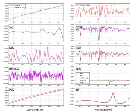
Fig. 1: Detailed intercomparison of a single OMI pixel (over Korea, IUPB-BIRA NO<sub>2</sub>: 3x10<sup>14</sup> molec/cm<sup>2</sup>, medium agreement).
