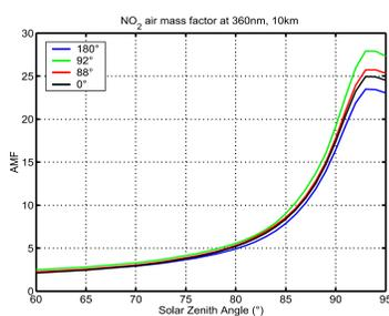
NO<sub>2</sub> AMF at 360nm. The AMFs increase with solar zenith angle, no big difference for the four directions. The zenith view direction have smaller AMFs.
