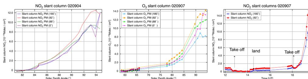
The left figure is the NO<sub>2</sub> time series on Sep. 7th. We can see the height character of AMAXDOAS measurement. When the Falcon is on the ground, the NO<sub>2</sub> slant columns are larger than in the air. During take off and landing the NO<sub>2</sub> slant columns are also changing with height. Are there some profile information?
