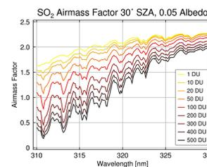
Figure: Airmass factors for SO<sub>2</sub> computed for different SO<sub>2</sub> columns located in a layer between 10 and 11 km
