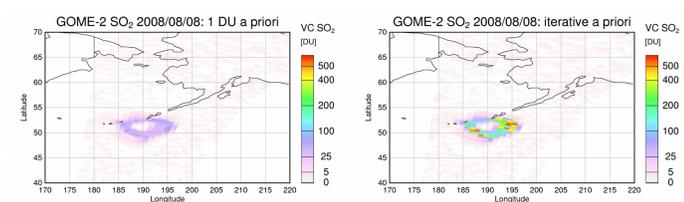
Figure: Effect of saturation correction on columns of the first day of observation of the Kasatochi eruption on August 8, 2008. Note the nonlinear colorscale. The estimate of the total SO<sub>2</sub> mass changes from 0.3 Tg to 1.35 Tg.
