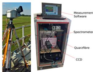
Fig 2: Telescope unit mounted on pan-tilt-head for azimuthal movement. Fig 3: Rack containing indoor parts.
