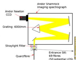
Fig 1: Sketch of the instrument's spectrometer.
