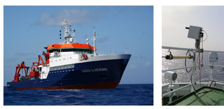
**Figure 1: Research vessel Maria S. Merian** A MAX-DOAS instrument was installed on board of the research vessel for the COPMAR project in October 2016.
