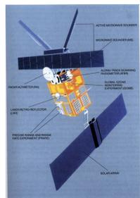
The Global Ozone Monitoring Experiment (GOME) and the SCanning Imaging Absorption spectroMETER for Atmospheric CHartography (SCIAMACHY) are two space borne nadir viewing grating spectrometers covering the spectral region from the UV to the NIR at moderate spectral resolution.
