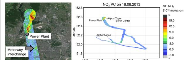
Figure: Strong variations of NO<sub>2</sub> amounts over Berlin and surroundings. Largest amounts are caused by power plant emissions, smaller scale NO<sub>2</sub> variations are also visible, e.g. around a motorway interchange and some industrial areas. NO<sub>2</sub> amounts in rural areas as well as above parts within Berlin City are substantially lower.
