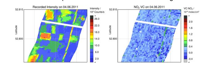
Figure: Measurement details from above motorway A1 showing the recorded intensity (left) and the NO<sub>2</sub> amount (right). The intensity is enhanced above the motorway and even more above bright fields west of the road. NO<sub>2</sub> amounts are slightly enhanced only above the motorway at (5±2)·10<sup>15</sup> molec/cm<sup>2</sup>.
