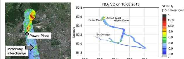
Figure: Strong variations of NO<sub>2</sub> amounts over Berlin and surroundings. Largest amounts are caused by power plant emissions, smaller scale NO<sub>2</sub> variations are also visible, e.g. around a motorway interchange and some industrial areas. NO<sub>2</sub> amounts in rural areas as well as above parts within Berlin City are substantially lower.
