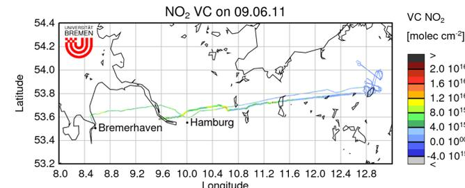
Figure: NO<sub>2</sub> amounts measured during a flight across Northern Germany with larger and strongly variable NO<sub>2</sub> amounts around 1·10<sup>16</sup> molec/cm<sup>2</sup> above and close to cities such as Hamburg, and consistently low values above remote, clean areas towards the East.
