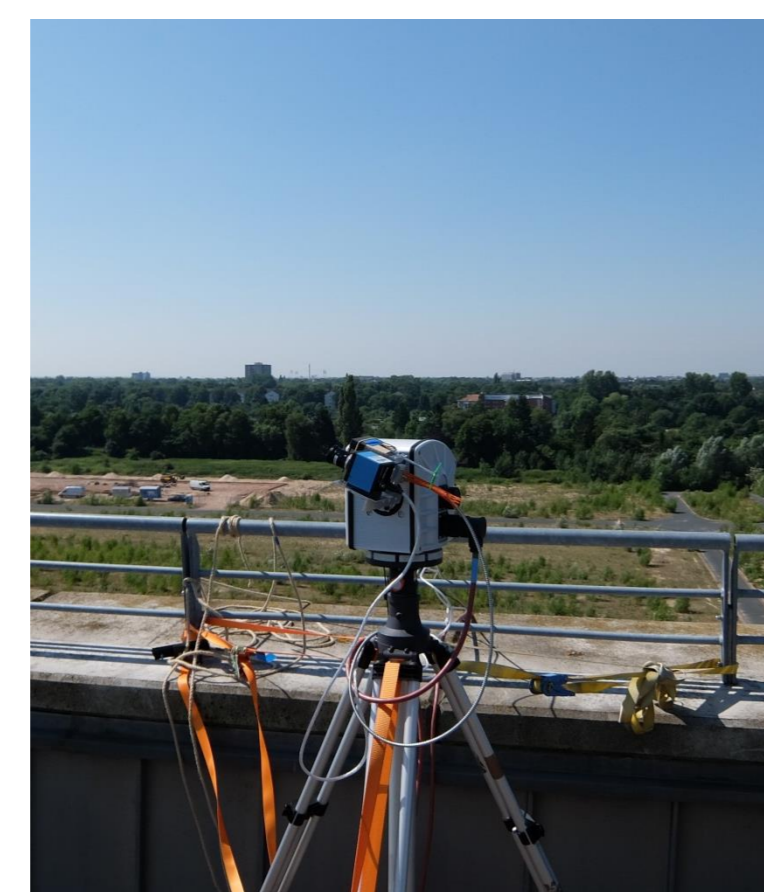
Fig 2: Entrance optic providing 35 elevations simultaneously mounted on pan-tilt-head for azimuthal movement.
