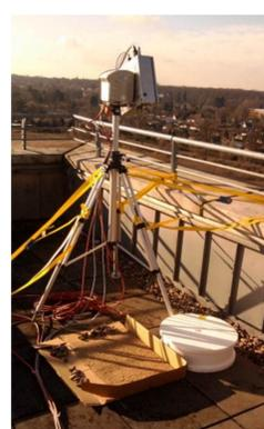
Figure: Experimental set-up on the roof of the IUP building with MAX-DOAS telescope on tripod and box with desert sand on the ground
