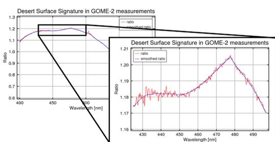
Figure: Logarithm of the ratio of two very close observations with different fitting residuals. Red is the original ratio with some residual Ring structures, blue the smoothed version used in the retrieval
