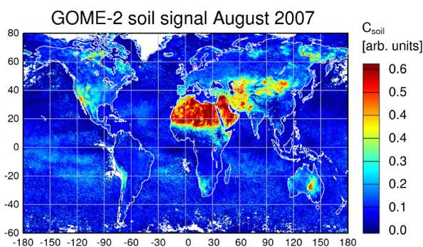
Figure: Average fitting coefficient for the empirical sand spectrum in one month of GOME-2 data. A cloud threshold of 20% has been used.
