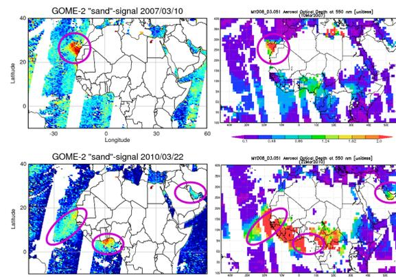
Figure: GOME-2 sand signal over the oceans (left) and MODIS AOD (right). Regions with enhanced sand signals are highlighted.
