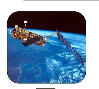
Atmospheric CHartographY) is an imaging spectrometer whose primary mission objectives are global measurements of trace gases in the troposphere and in the stratosphere. The solar radiation transmitted, backscattered and reflected from the atmosphere is recorded at relatively high resolution (0.2 nm to 1.5 nm) over the range 240 nm to 1700 nm, and in selected regions within 2.0 µm and 2.4 µm. SCIAMACHY has a global coverage of 6 days with a spatial resolution of 60kmx30km.
