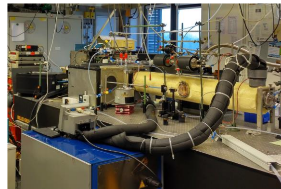
Figure 49: Echelle spectrometer setup with insulated double wall absorption cell for ozone absorption cross-section measurements at cold temperatures.
