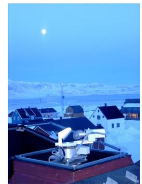
Figure 1: Lunar absorption measurements in the Arctic at the AWIPEV research base in Ny-Ålesund, Spitzbergen. The solar tracker in the picture directs the lunar light into the building where a Fourier Transform InfraRed (FTIR) spectrometer is used to determine the concentrations of CO<sub>2</sub> and CH<sub>4</sub> in the atmosphere from characteristic absorptions in the lunar light.
