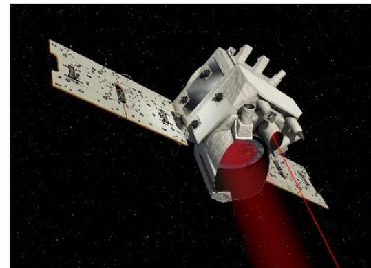
Figure 49: Artist's conception of the MERLIN satellite which will monitor atmospheric methane using a lidar instrument. (CNES/Illustration D. Ducros)
