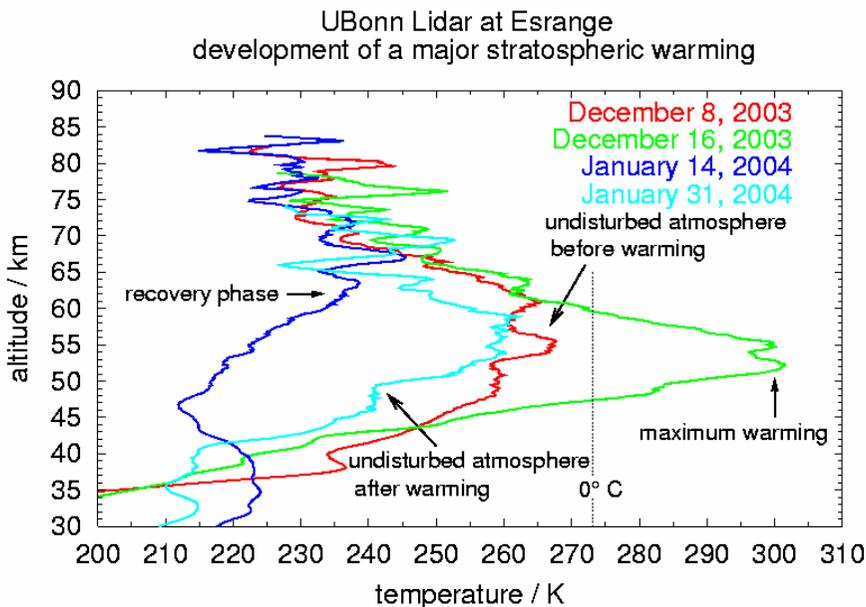
Fig. 4: The different stages of a major stratospheric warming observed with the U. Bonn lidar at the Esrange.
