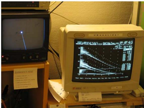
Fig. 3: Operator console of the U. Bonn lidar. A CCD-camera observes continuously the laser beam in the atmosphere (left monitor). The bright spot is from a tenuous low altitude cloud. The current measurement raw-data are shown on the right monitor.
