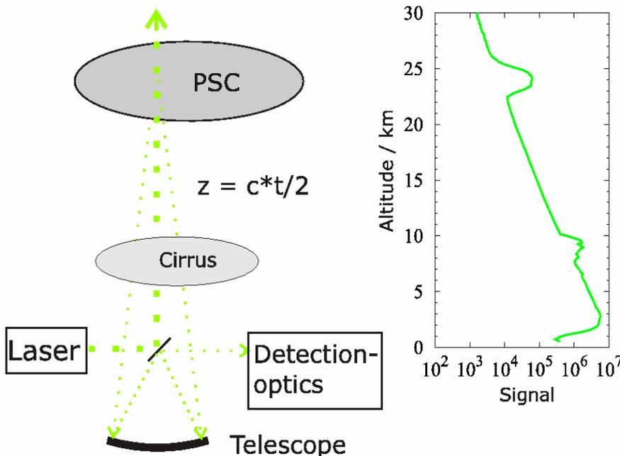
Fig. 2: Principle of a Rayleigh/Mie/Raman lidar experiment (left side) and the resultant raw-data profile (right side). The molecular signal drops of exponentially with altitude. The signal enhancements at 8 km and 24 km altitude are caused by clouds. The decrease of the signal below 3 km altitude is caused by an incomplete overlap between the laser beam and the field of view of the telescope.
