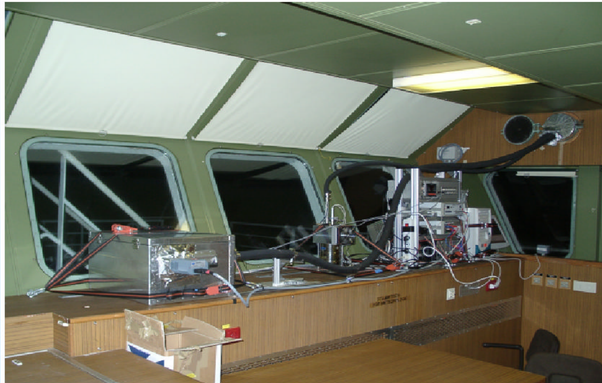
Figure 3-4: Indoor set-up with the UV and VIS detecting units, the rack with the control units, the computer and the rubber hoses being introduced through a cable door.
