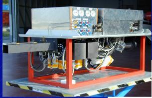
Simultaneous measurement in two parallel measurement ducts yields two independent Cl and Br measurments.
