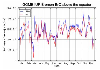
**Figure 5:** GOME BrO vertical columns above the equator for 1996 and 1997 as derived by the IUP Bremen. Again, similar structures seen in Figures 1 - 4 appear, however with a different amplitude and not at the same time of the year.
