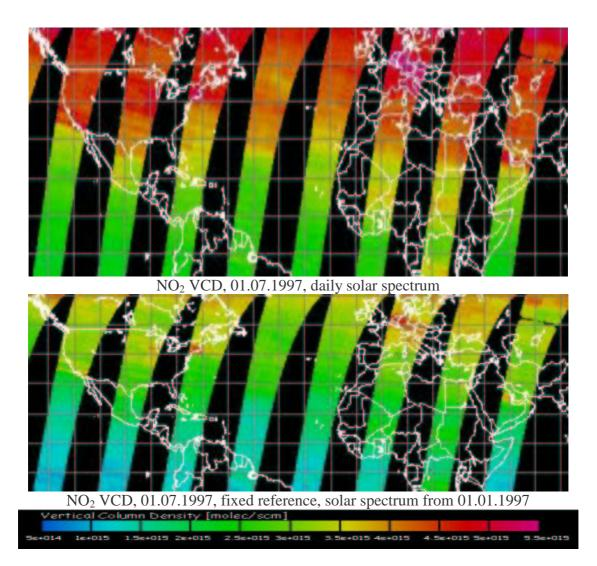
**Figure 6:** Examples GOME NO<sub>2</sub> maps for a day (01.07.1997) with a large uncertainty introduced by the spectral structures caused by the diffuser plate. Especially in the Tropics the difference between the evaluation with fixed or daily reference spectrum can be large (up to about 100%).
