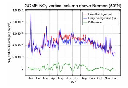
**Figure 2:** GOME NO<sub>2</sub> vertical columns above Bremen as derived with a daily irradiance spectrum (lv2 product) and a fixed background spectrum. The difference between the two evaluations is the structure introduced by the diffuser plate, but divided by the airmass factor applied to the slant columns.
