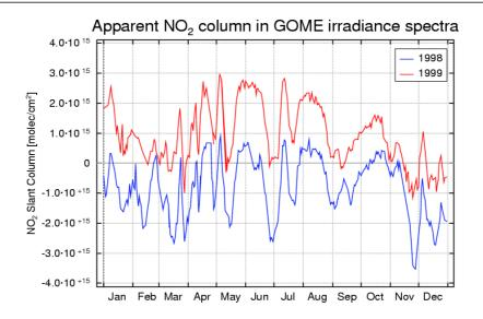
**Figure 3:** Apparent NO<sub>2</sub> slant column when applying the standard NO<sub>2</sub> fit to all GOME irradiance spectra, using one arbitrarily chosen solar spectrum as background. Small and random columns are expected, but large and systematic variations are found. The similarity between the structures found in this test and in Figures 1 and 2 are obvious.
