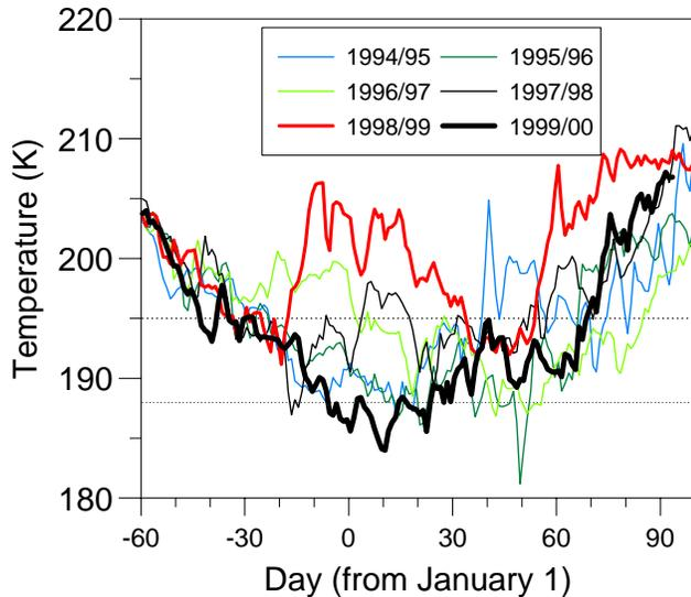
**Figure 1.** Minimum temperatures at the 46 hPa level from UKMO analyses for the last 6 winters. The winter of 1999/2000 was characterized by very low temperatures during December and January and a long period of temperatures below the possible PSC formation temperature.
