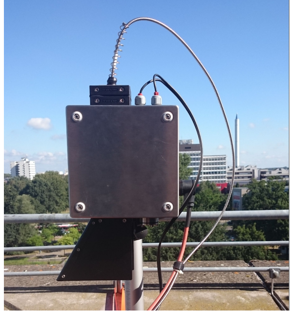
(b) Bend protection and strain relief of the light fibre
