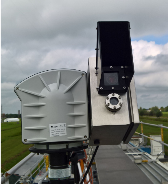
(a) Mounting of filter glass at the telescope
