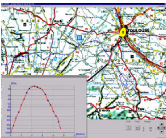
Fig. 3: Flight trajectory (left) and SCIAMACHY overpass (right) for TRIPLE flight on 24.09.02 from Aire sur l'Adour (France), and on 06.03.03 from Kiruna (Sweden). Flight parameters were optimized for satellite overpass on balloon descent, where best contamination-free measurements can be made.
