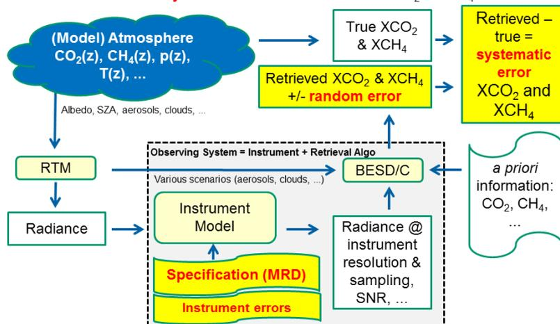
Fig. 2: Framework for the generation of simulated CarbonSat observations with the goal to estimate random and systematic XCO<sub>2</sub> and XCH<sub>4</sub> retrieval errors for different conditions. As radiative transfer model (RTM) SCIATRAN [7] is used. BESD/C is the CarbonSat Level 1 to 2 retrieval algorithm under development at Univ. Bremen.
