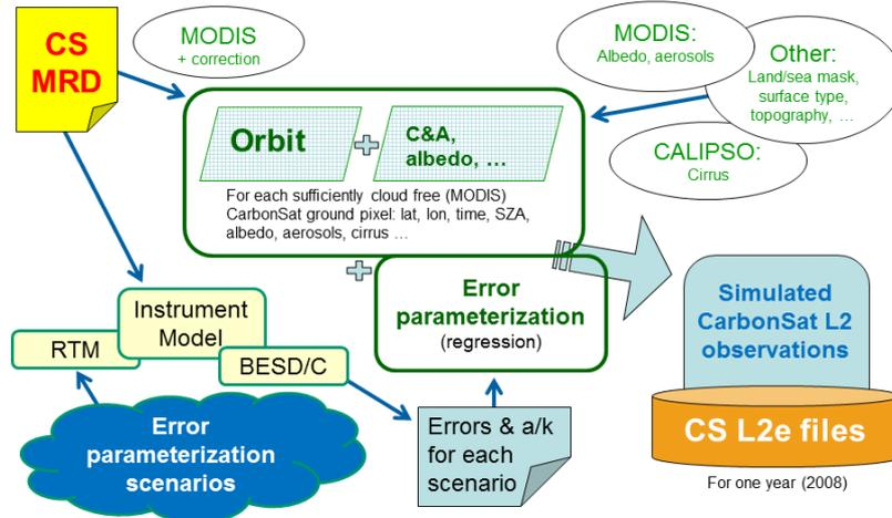
Fig. 4: Framework for the generation of one year of simulated CarbonSat (CS) observations, i.e., for the generation of the CarbonSat Level 2 error (L2e) files. MRD refers to CarbonSat's Mission Requirements Document [4]. a/k stands for averaging kernels, which are also computed and parameterized, and C&A means Clouds & Aerosols.
