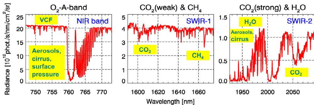
Fig. 1: Typical CarbonSat radiance spectrum as measured in the three spectral bands NIR, SWIR-1 and SWIR-2 (see also Tab. 1).
