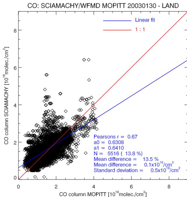
Figure 4. Comparison of the column-averaged CO concentrations from the WFM-DOAS algorithm and those measured by the MOPITT measurements for January 30, 2003. Note that the WFM-DOAS data have been multiplied by a factor 0.5 as explained in [9]. Only pixels over land are shown.
