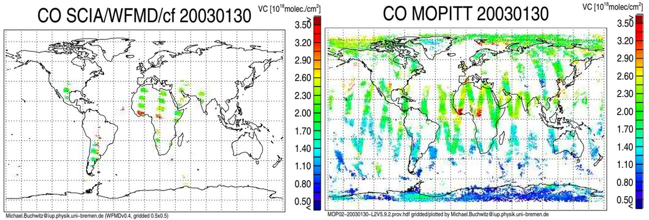
Figure 3. Left: CO total columns from the WFM-DOAS retrieval algorithm for January 30, 2003. Only cloud-free pixels are shown. Right: The corresponding CO total columns as measured with the MOPITT instrument (from: <http://www.eos.ucar.edu/mopitt/data/plots/mapsv3.html>). Note that both figures use the same vertical scale (from: [9]).
