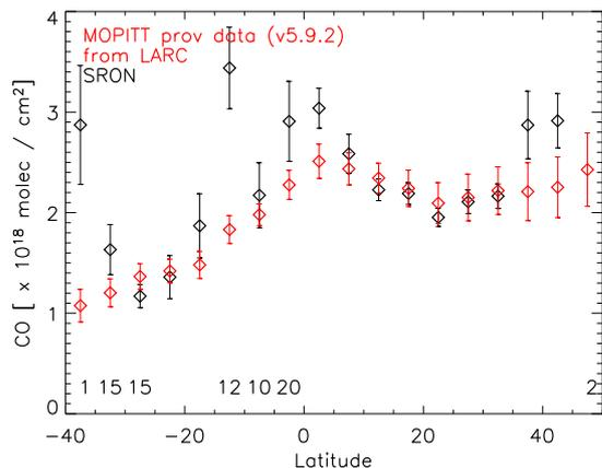
Figure 6. Comparison of the monthly CO total columns for February 2004 as presented in Fig. 5, where all data within a five degree latitude bin have been averaged (see text). The black diamonds denote the IMLM CO total columns, the red diamonds the corresponding MOPITT data. Only cloud-free pixels with instrument noise related errors  $< 1.5 \times 10^{18}$  molec/cm<sup>2</sup> have been included. The error bars denote the instrument noise related errors only.
