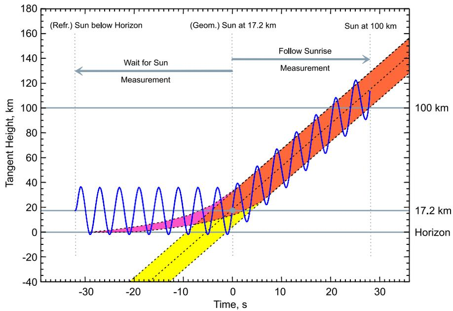
Fig. 5: Solar occultation scan strategy. Pink: Size of refracted sun. Yellow: Size of geometrical sun.
