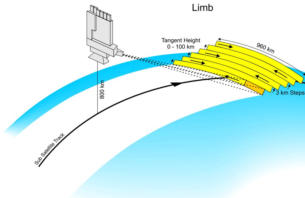
Fig. 4: Nominal limb scan mode of SCIAMACHY.
